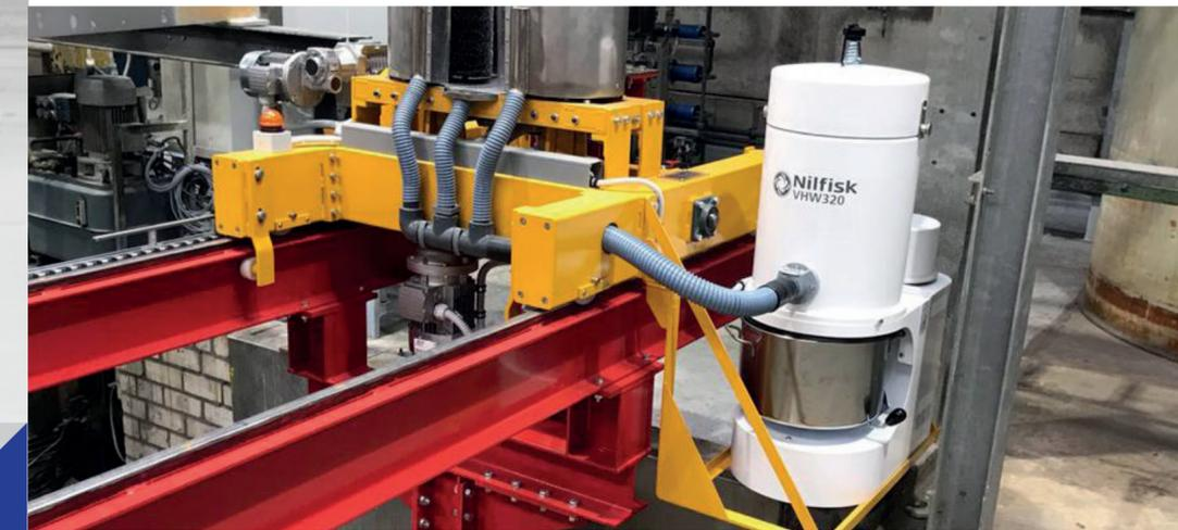
**Machine**, totally designed by **Monti Engineering**, which carries out a mechanical removal of oxide and salts from the handling bars surface.
