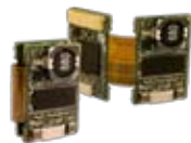
CBC Single-axis miniature controller with a built-in amplifier
