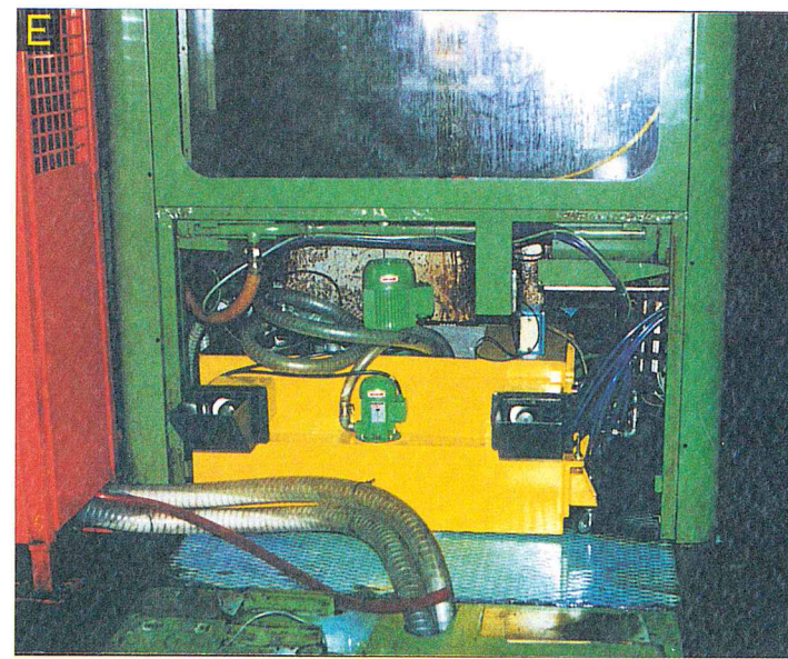
Prefiltration unit of the lubricating-cooling fluid connected directly to two screw conveyors installed in a work centre.
