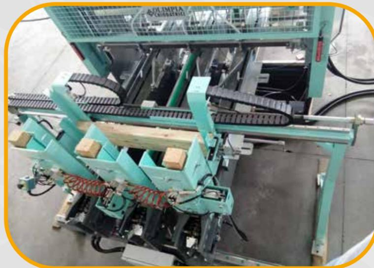
**TSL - Nail Clipper For Bridges Assembly**
